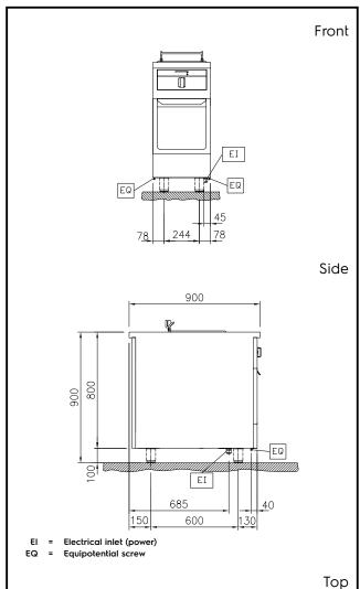
Electric Supply voltage: 400 V/3N ph/50/60 Hz Total Watts: 10 kW **Key Information:** Number of wells: Usable well dimensions (width): 240 mm Usable well dimensions 225 mm (height): Usable well dimensions 380 mm (depth): Well capacity: 12 lt MIN; 14 lt MAX Thermostat Range: 100 °C MIN; 180 °C MAX External dimensions, Width: 400 mm External dimensions, Depth: 900 mm External dimensions, Height: 800 mm Net weight: 75 kg On Base;One-Side Configuration: Operated
